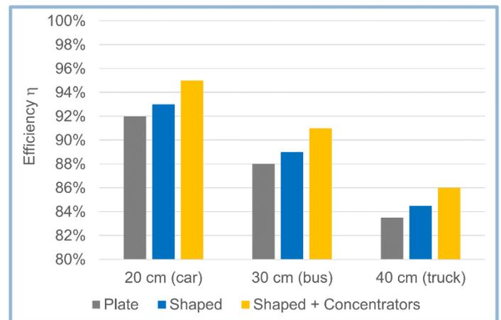
Fig. 5 Transmitter-pickup coil distance for different electrical vehicles
